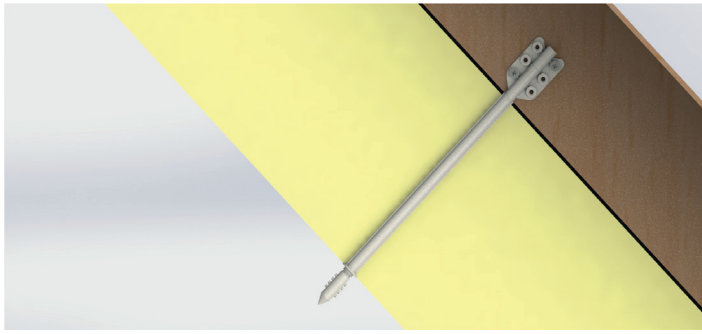
1. Fix the hanger on the frame
