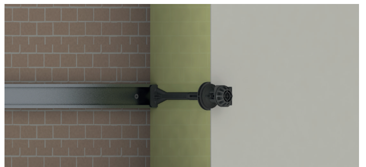
6. Adjust the head of the support then clip it
